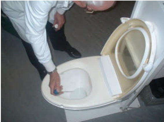
CREH laboratory introducing E.coli to a Propelair prototype to test bacterial aerosol
